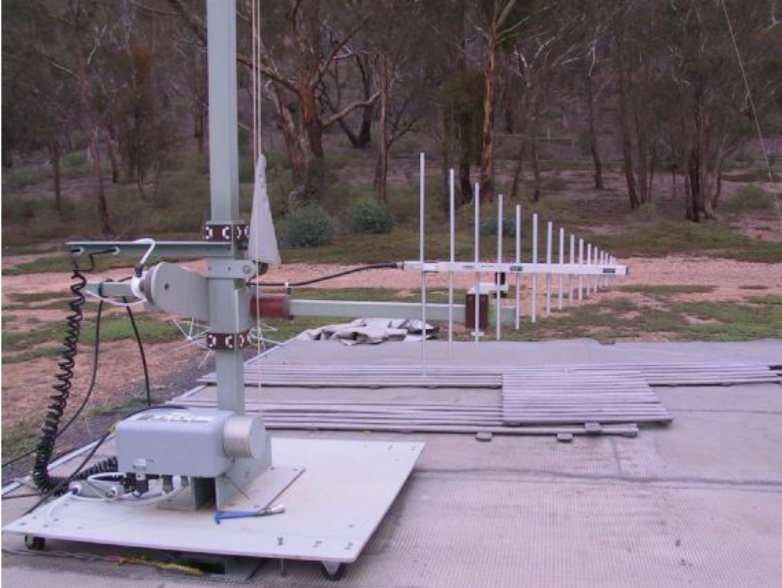
Figure 25 – Log Periodic antenna used for testing 230MHz-1GHz (Equipment courtesy of EMC Technologies Pty Ltd)
