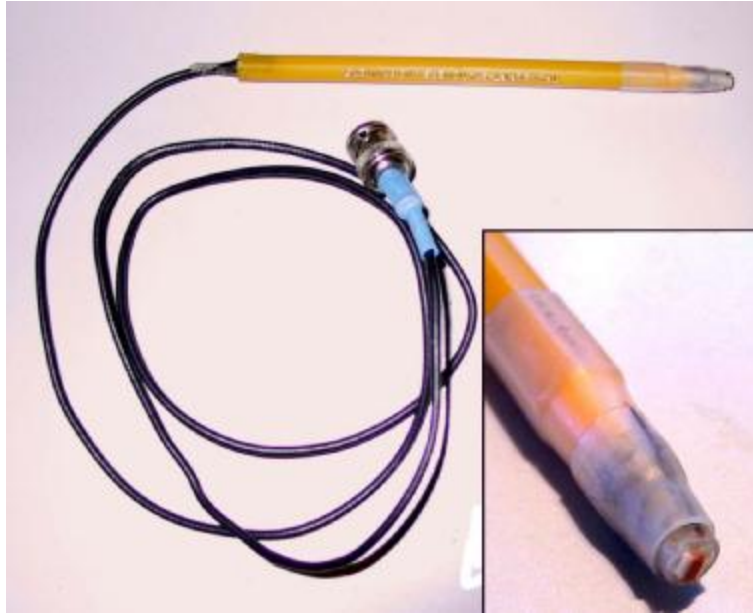
Figure 1 – A home made inductive probe. (Note the line drawn near the tip to indicate the plane of the coil)
