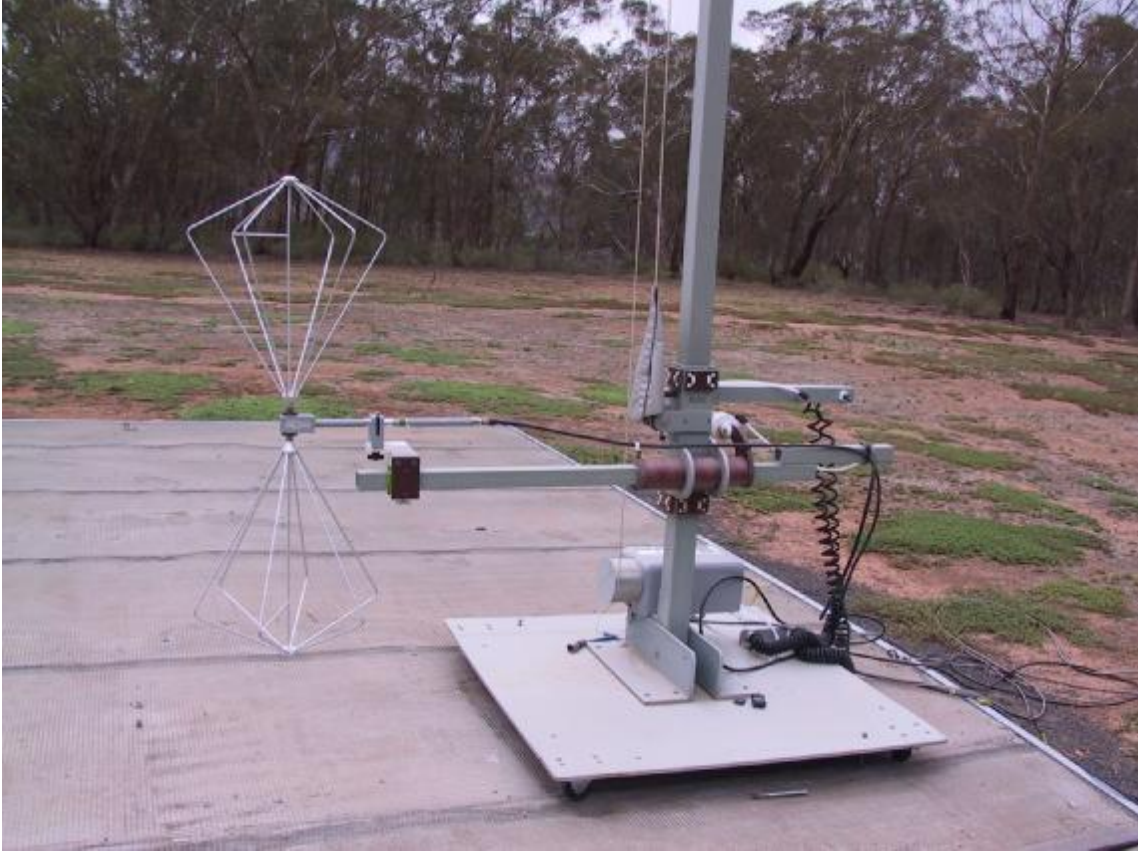
Figure 24 – A broadband antenna used for testing to 230MHz. Antenna height is remotely adjustable up to 4 metres. (Equipment courtesy of EMC Technologies Pty Ltd)
